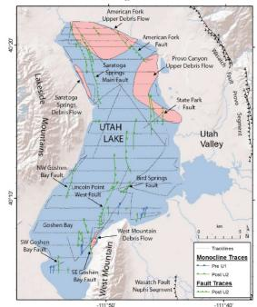
**Figure 3.** Seismic faults and debris flow deposits in Utah Lake (Dinter 2014).
